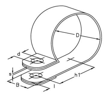
$\begin{array}{ll} d & = 5.3 \\ \text{Diameter D} = 15 \\ \text{h1} & = 14.3 \\ \text{I} & = 5.0 \\ \text{s} & = 0.5 \\ \text{Width B} & = 12 \\ \end{array}$
